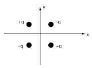
The first thing we need to do is define the position vectors for each charge and then find the dipole moment about the origin for each charge and take the vector sum.
