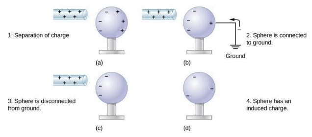
Charging by induction using a ground connection. (a) A positively charged rod is brought near a neutral metal sphere, polarizing it. (b) The sphere is grounded, allowing electrons to be attracted from Earth's ample supply. (c) The ground connection is broken. (d) The positive rod is removed, leaving the sphere with an induced negative charge.
