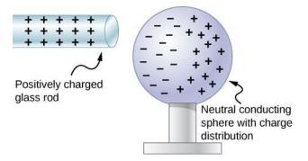
Induced polarization. A positively charged glass rod is brought near the left side of the conducting sphere, attracting a negative charge and leaving the other side of the sphere positively charged. Although the sphere is overall still electrically neutral, it now has a charge distribution, so it can exert an electric force on other nearby charges. Furthermore, the distribution is such that it will be attracted to the glass rod.
