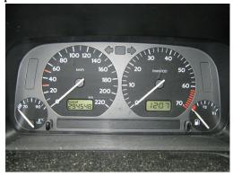
The fuel and temperature gauges (far right and far left, respectively) in this 1996 Volkswagen are voltmeters that register the voltage output of "sender" units, which are hopefully proportional to the amount of gasoline in the tank and the engine temperature. (credit: Christian Giersing)
